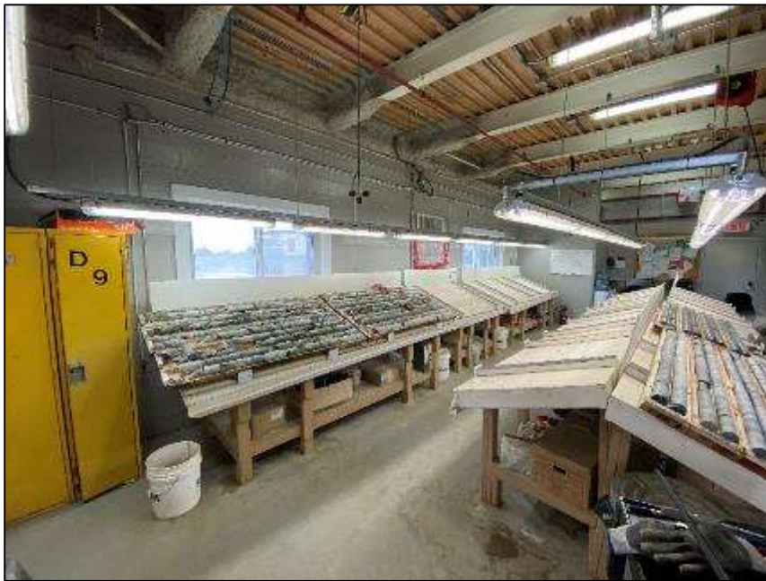
Figure 12-10: OR-22-55 and OR-22-56 drill core (Watson Lake Group sericitized rhyolites at end of OR-22-55 (right) and chlorite altered hanging wall basalts at top of OR-22-56 (left))
