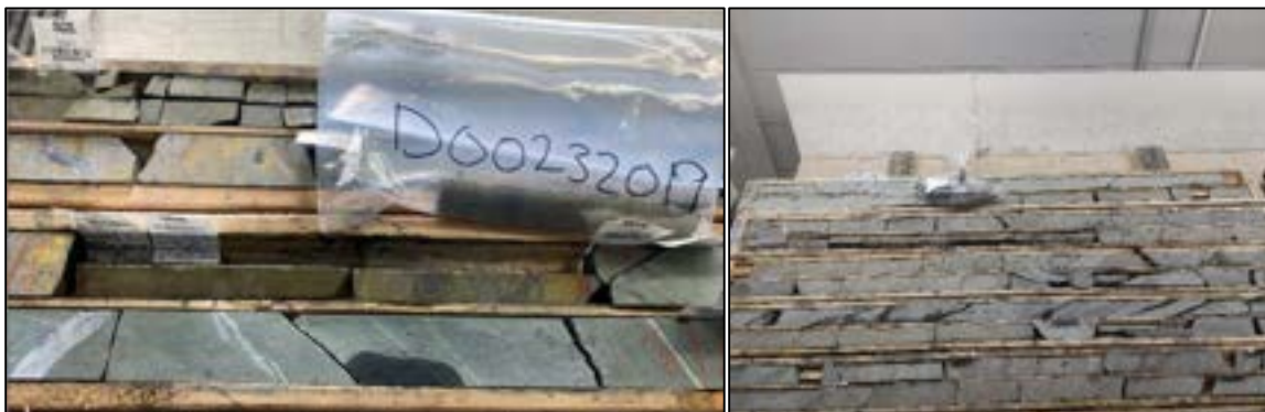
Figure 12-15: Example of IW quarter core check samples collected in 2022 (left) and 2024 (right)
