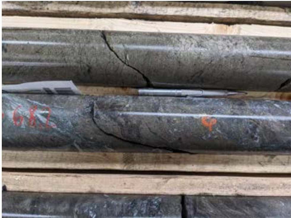
Figure 12-4: Sphalerite-chalcopyrite-pyrite mineralized interval – PD1-23-47 at 68 m (PD1 deposit)
