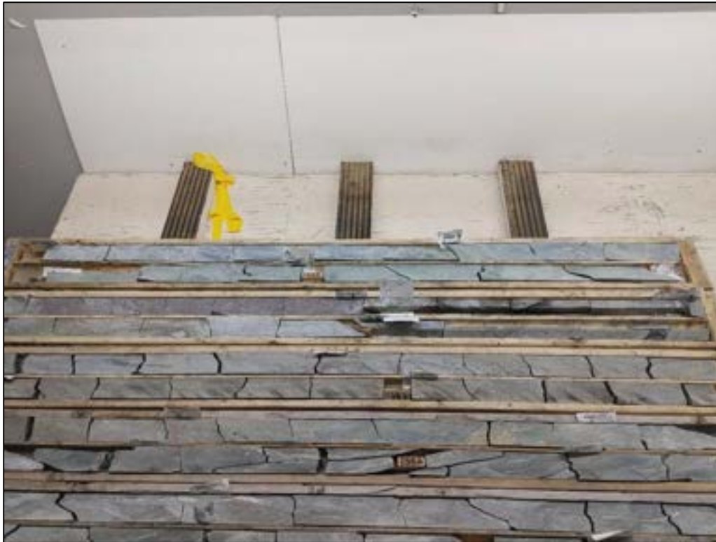
Figure 12-12: MCL-13-31W2 (characterized as pipe alteration with semi-massive to massive sulphide mineralization of chalcopyrite and red-brown sphalerite intermixed with pyrite and pyrrhotite)
