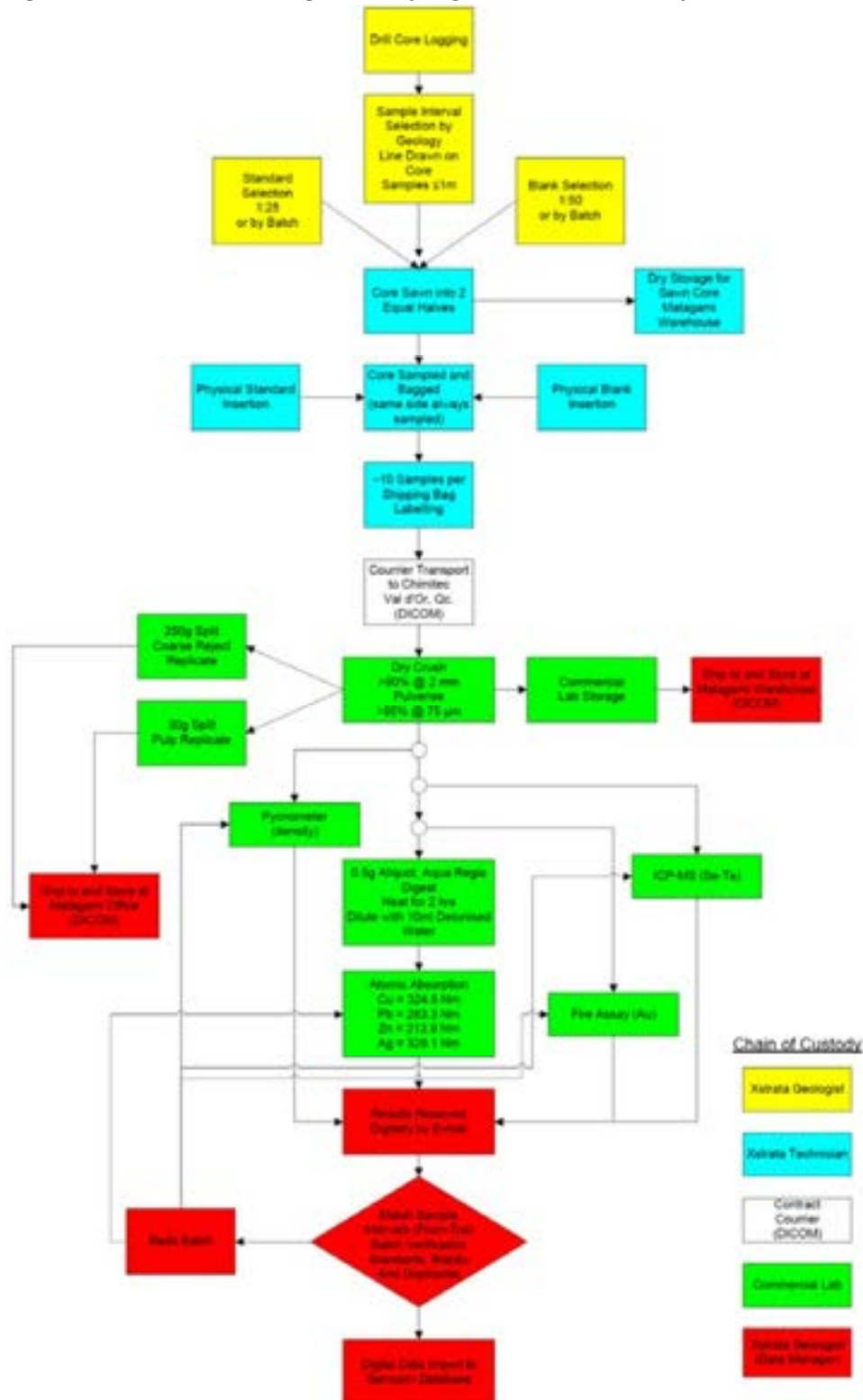
Figure 11-1: Glencore Matagami sampling flowsheet – PD1 deposit
