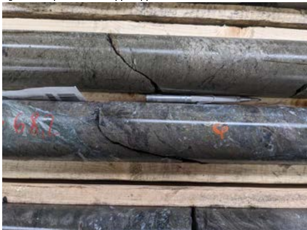
Figure 12-4: Sphalerite-chalcopryrite-pyrite mineralized interval – PD1-23-47 at 68 m (PD1 deposit)
