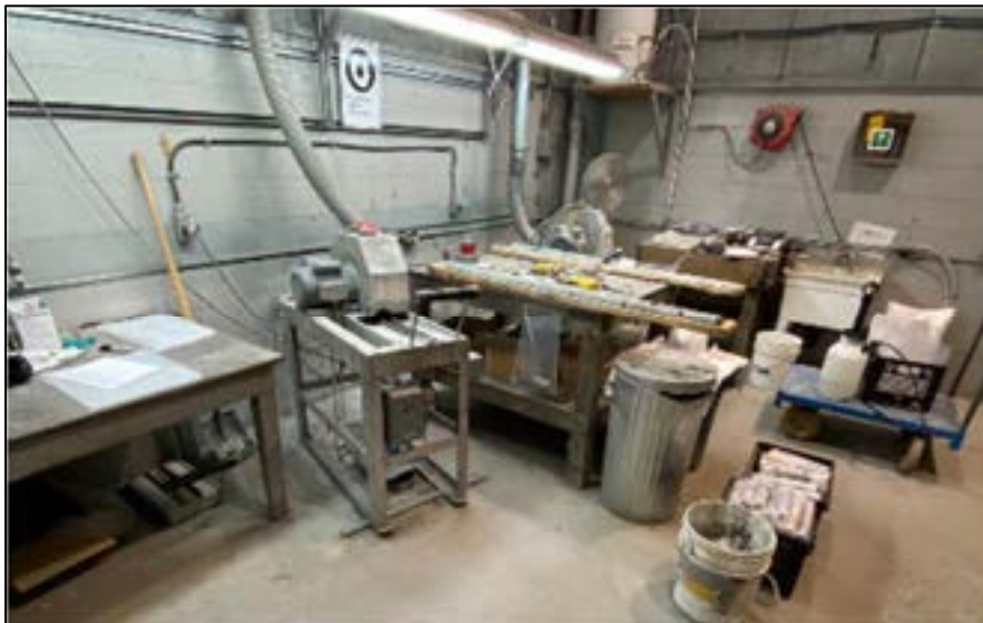
Figure 12-13: Project core cutting facility used for the IW quarter core check sample program
