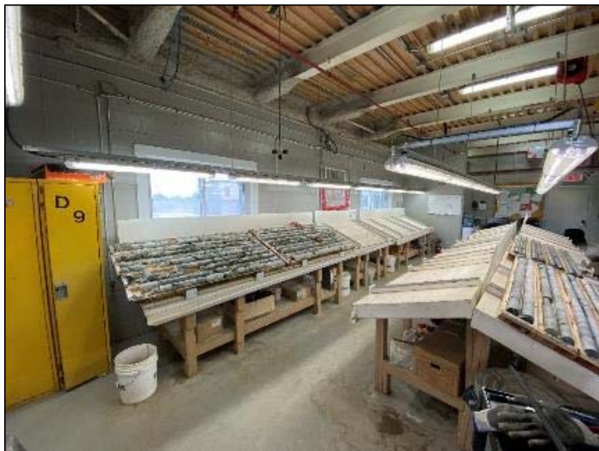
Figure 12-9: OR-22-55 and OR-22-56 drill core laid out for inspection (Watson Lake Group sericitized rhyolites at end of OR-22-55 (right) and chlorite altered hanging wall basalts at top of OR-22-56 (left))
