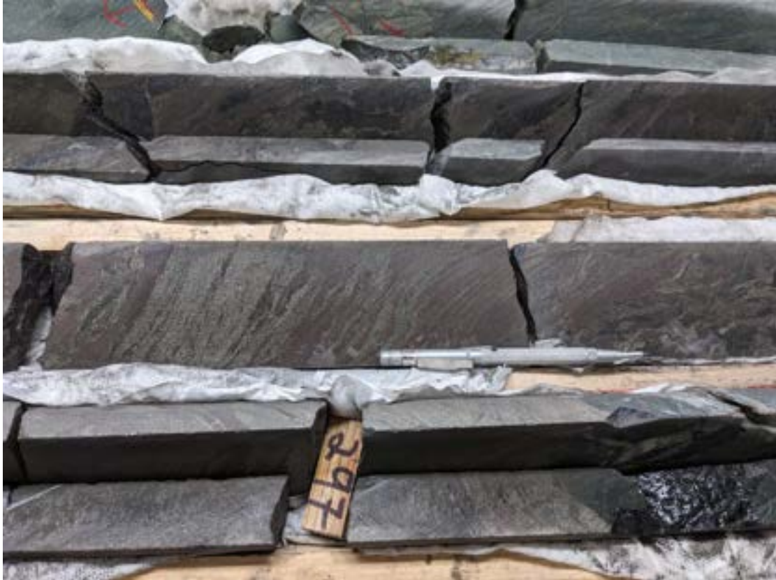
Figure 12-3: Sphalerite-pyrite-magnetite mineralized interval – GCB-23-107 at 296 m (Caber deposit)
