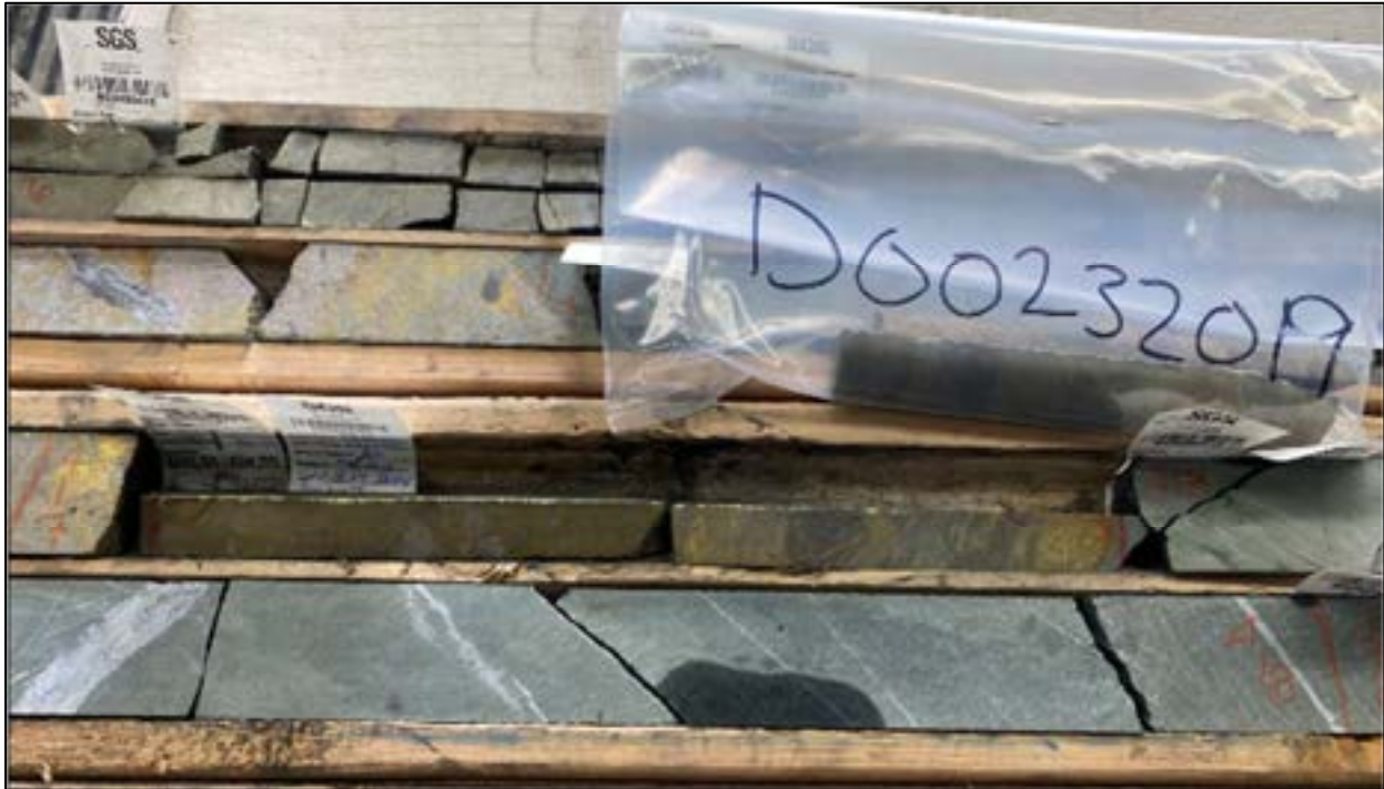
Figure 12-12: Example of IW quarter core check sample
